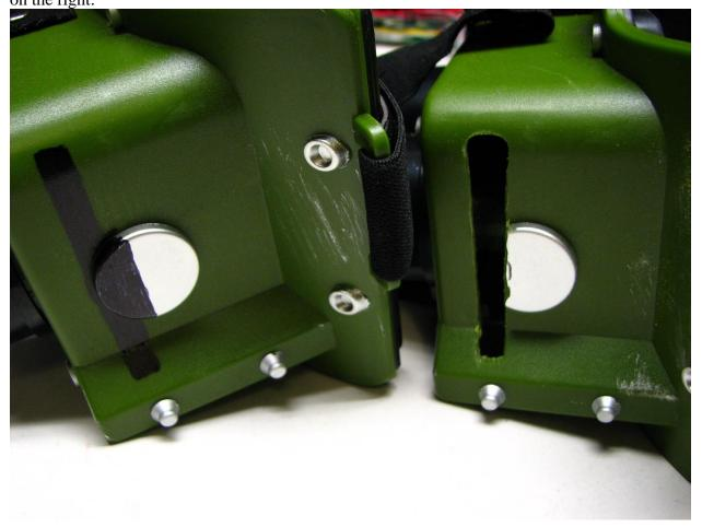
On the left, I just used a sharpie to make the knob and case disappear in the slot. On the right I cut out the slot so that the opening would go down into the goggles. The depth from the top of the right-side film opening part is about 1 inch deep when the case and knob are cut out of the way.
