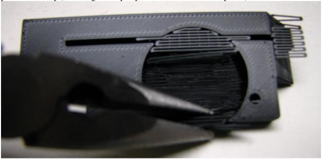
The slot should be cleared and there may be some extra material in one of the mounting holes. Here is the cleaned-up part:
