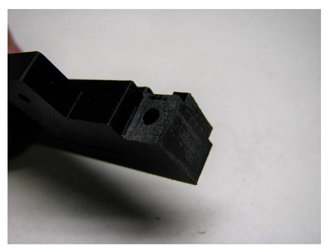
The left side display head (#8) has scaffolding to support the pivot mechanism, both on the outside and the inside where the screws will be placed. Again, I like using some needle nose pliers to grasp the scaffolding and twist and pull it away from the part.
