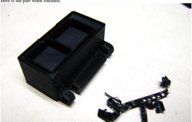
If you have some leftover scaffolding inside the holes, you can use a smaller drill bit to remove the scaffolding. Take care not to make the holes larger, since you do want to make sure the screws will hold the parts together. I use a 1/16" bit if clearing out is needed.
