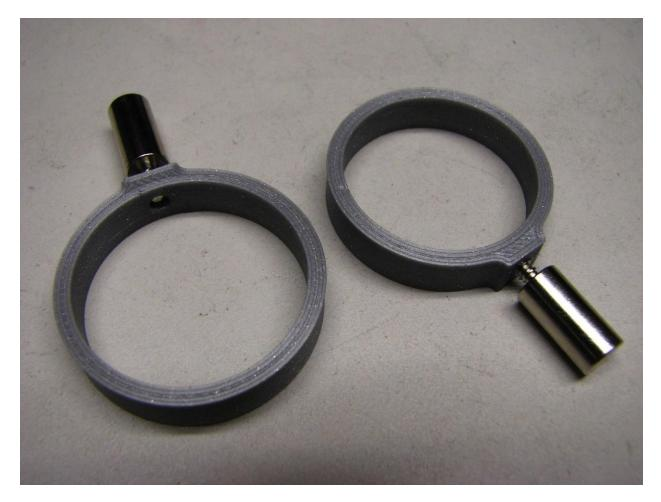
The rings can go on either way and once mounted they do not move like the larger rings knob sections of the goggles can. Orient the posts in the desired direction before you slide them on.
