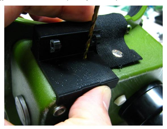
Press and hold the base while you drill the second hole. Then screw in the second black screw (#10). Now the base is attached to the goggles,
