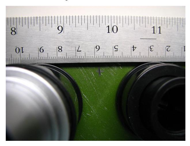
Drill a 5/16" hole, test fit the part and then put a small amount of glue in the hole edges (I used super glue) and hold the part in place.
