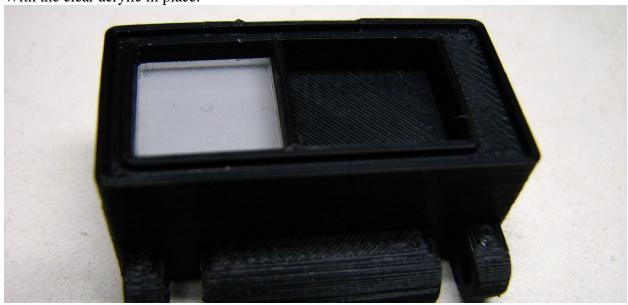
Do the same with the black acrylic piece: test fit by placing it vertical in each direction to make sure it is not overly tight, sand edge if needed, glue if you must then peel off the protective layers and press into place.
